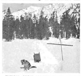
TYPICAL SNOW COURSE showing sampling tube and scales. The scales record water content of snow in tube. In foreground is surveyor's dog companion and heavy pack.
