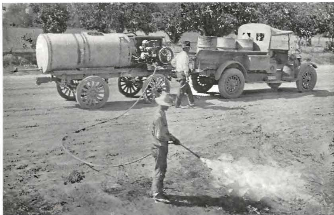
SPREADING POISON for the Puncture Vine, this outfit of truck and trailer equipped with tank and spray pump is being used in an earth sterilization experiment.
