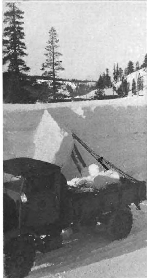
HIGHWAY SNOW FIGHTERS in action—The top pictures show front and rear views of one of the large railroad type rotary plows. The operating end is at the rear of the machine which backs into the drifts. Lower left is a slice bar mounted on a truck. At right is a V-plow with side wing.
