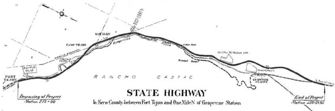
SKETCH MAP showing Grapevine Grade realignment. Heavy black line indicates new highway.
