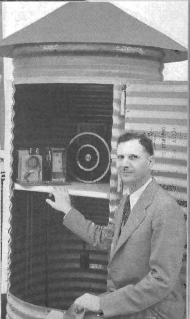
ON GUARD in little shelter houses along 13 California streams is this Ingerson automatic radio stream gage signal apparatus that sends out warnings of flood dangers. Front and rear views of the gage keying device and transmitter are shown in pictures 1 and 2 and inventor Irvin M. Ingerson, associated hydraulic engineer of the Division of Water Resources is shown with the installation in No. 4.
