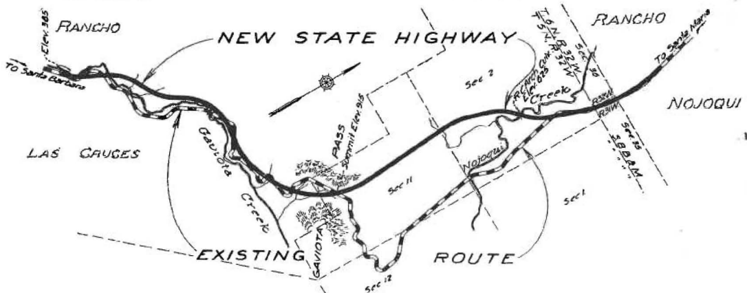
NEW NOJOQUI GRADE location is shown by heavy black line, old route by dotted line
