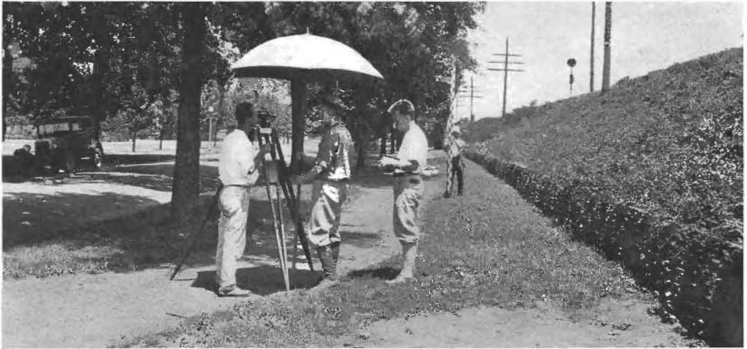
GEODETIC SURVEY LEVELING PARTY. The umbrella is to protect the instrument, not the observer.
