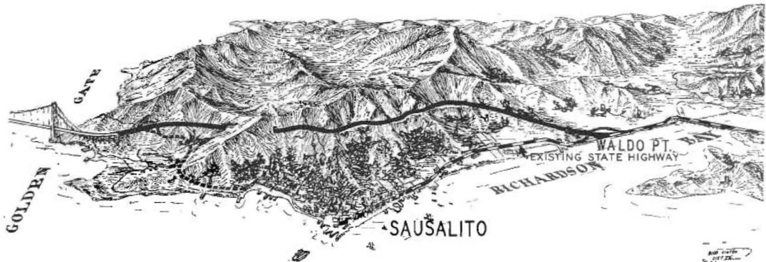
SKETCH OF STATE HIGHWAY Marin approach route showing location of tunnel through Sausalito Hills.
