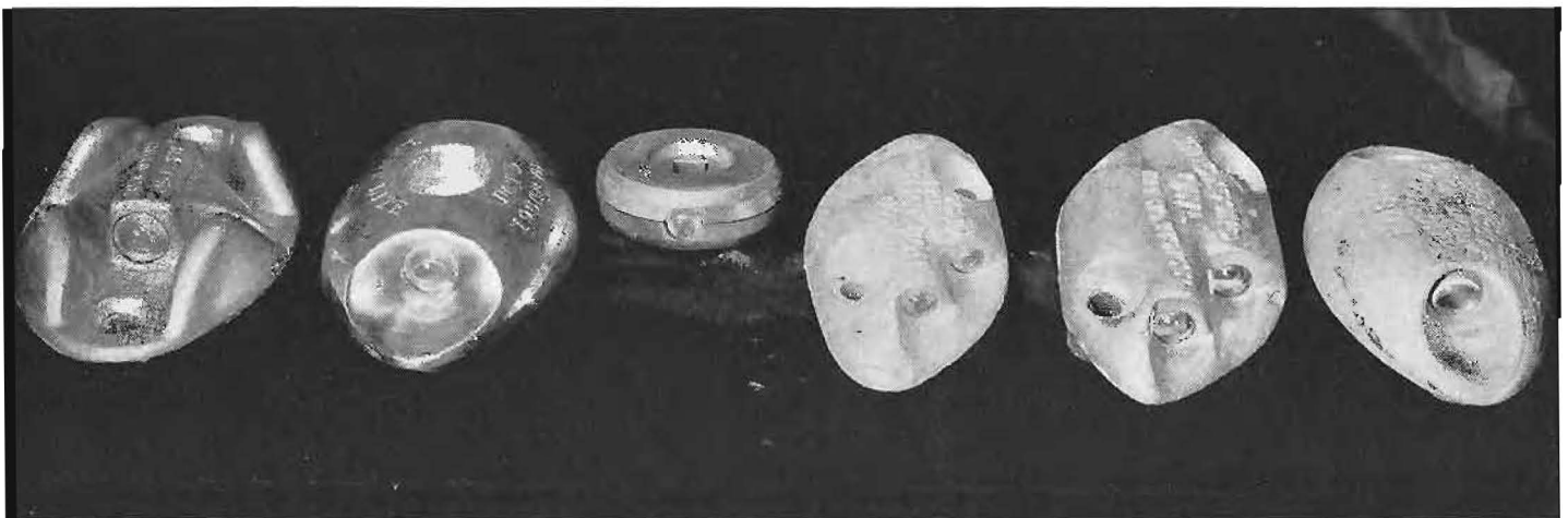
Types of reflectorized road buttons with which the Division of Highways is experimenting to test durability, visibility and maintenance cost. Replacement of buttons smashed or dislodged by heavy traffic and necessity for frequent removal of dust and mud accumulations are factors.
