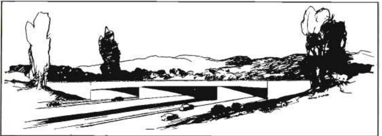
Proposed continuous concrete span structure carrying Hough Street over Arroyo Seco Parkway. Length 289 feet.
