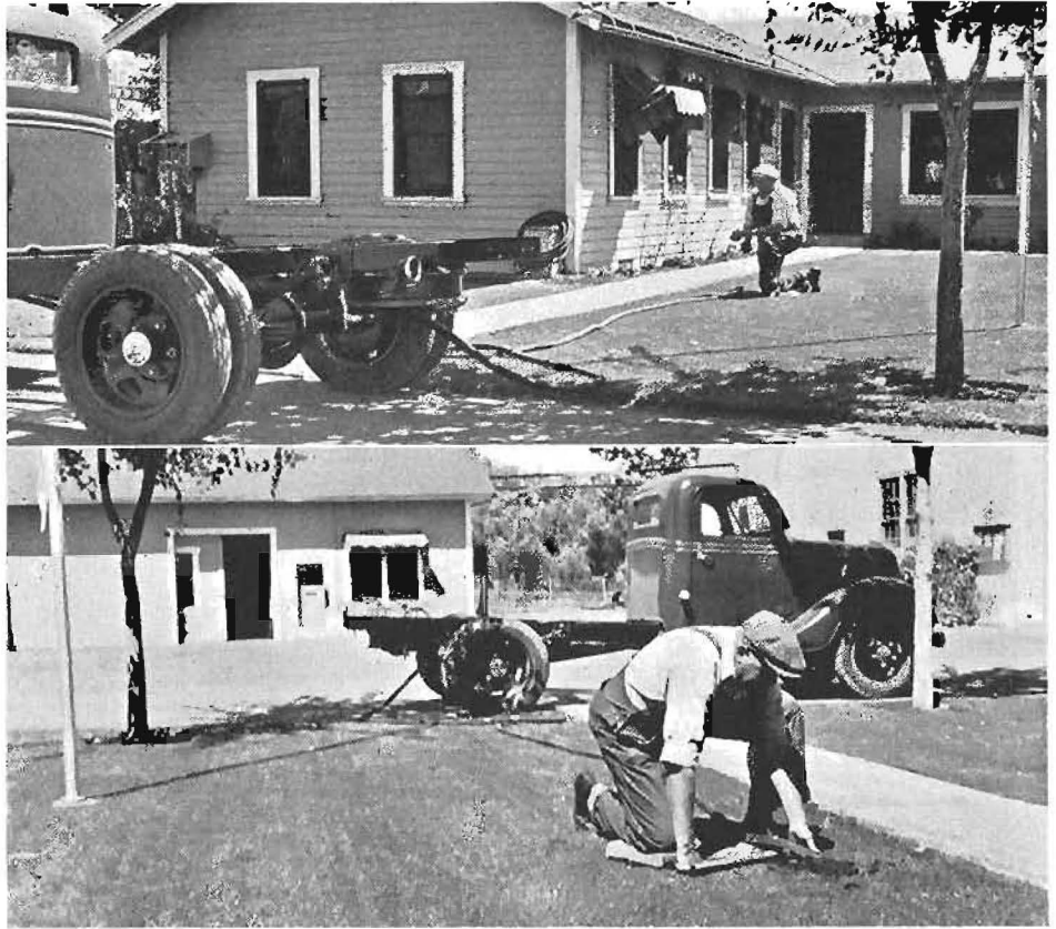
These pictures illustrate how moles were exterminated with monoxide gas by attaching one end of a hose to the exhaust pipe of a Division of Highways truck and poking the other end into mole hills.
