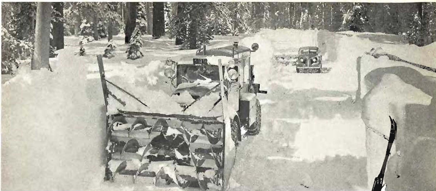
This is type of auger blower rotary snow plow, nine of which Division of Highways has added to its snow removal equipment for work in mountains this winter.
