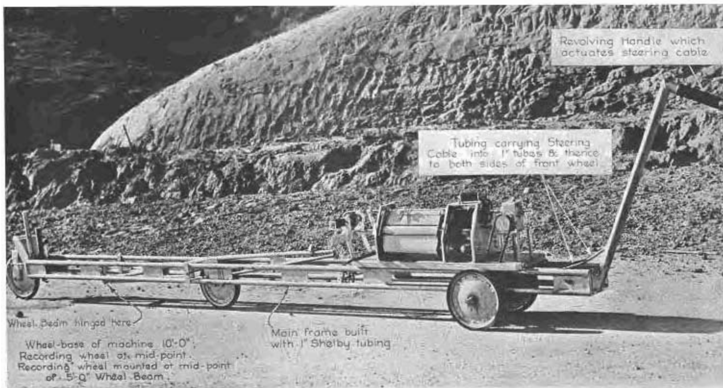
General view of newly designed Viagraph, a road surface meter machine equipped with recording attachments developed by highway engineers.
