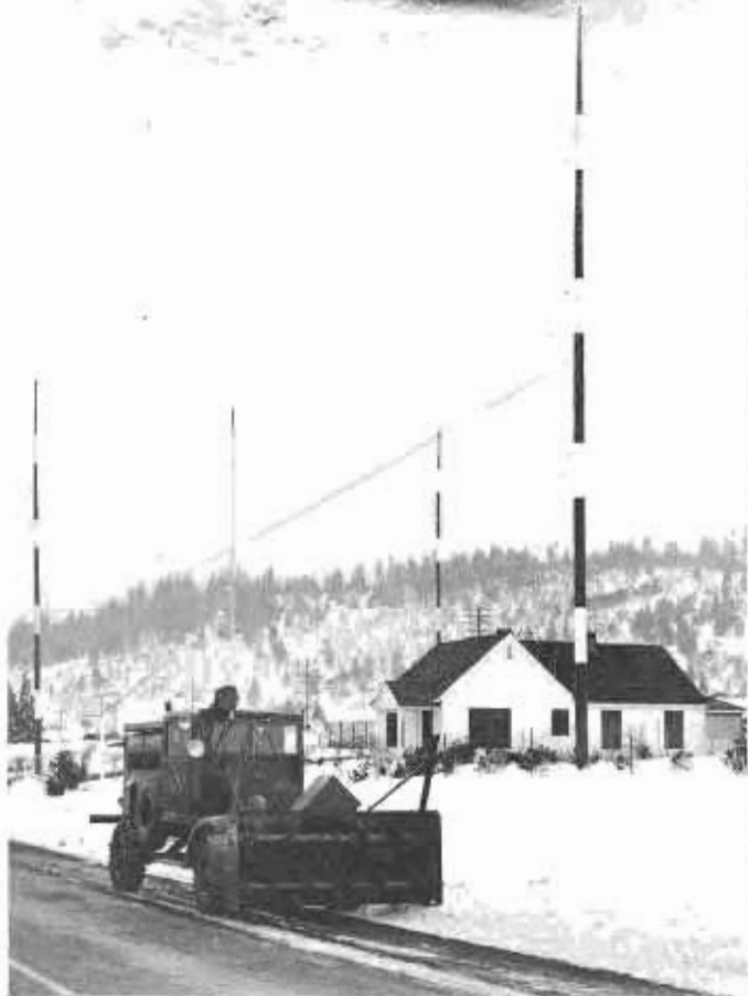
Upper left—Radio equipped snow plow with antenna raised working in isolated mountain section of Shasta County. Upper right—Foreman R. E. Frost in Shasta City maintenance station, KATR (lower left), transmitting instructions to plow operator (lower right), who hears and talks over loud speaker equipment in front of him.
