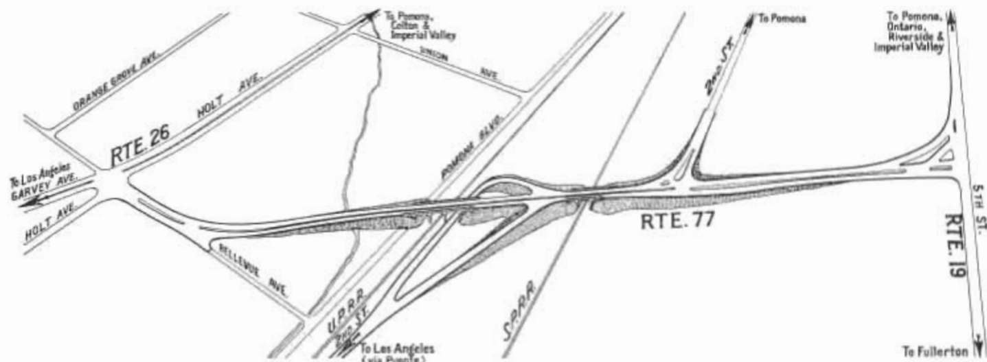
Grade separations over adjacent railroads and a city street on State Route 77 connected by channelized ramp approach system.
