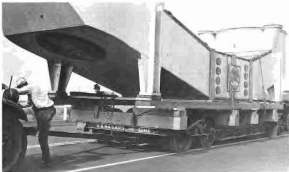
Largest parts were moved on 4-axle low bed trailer.
