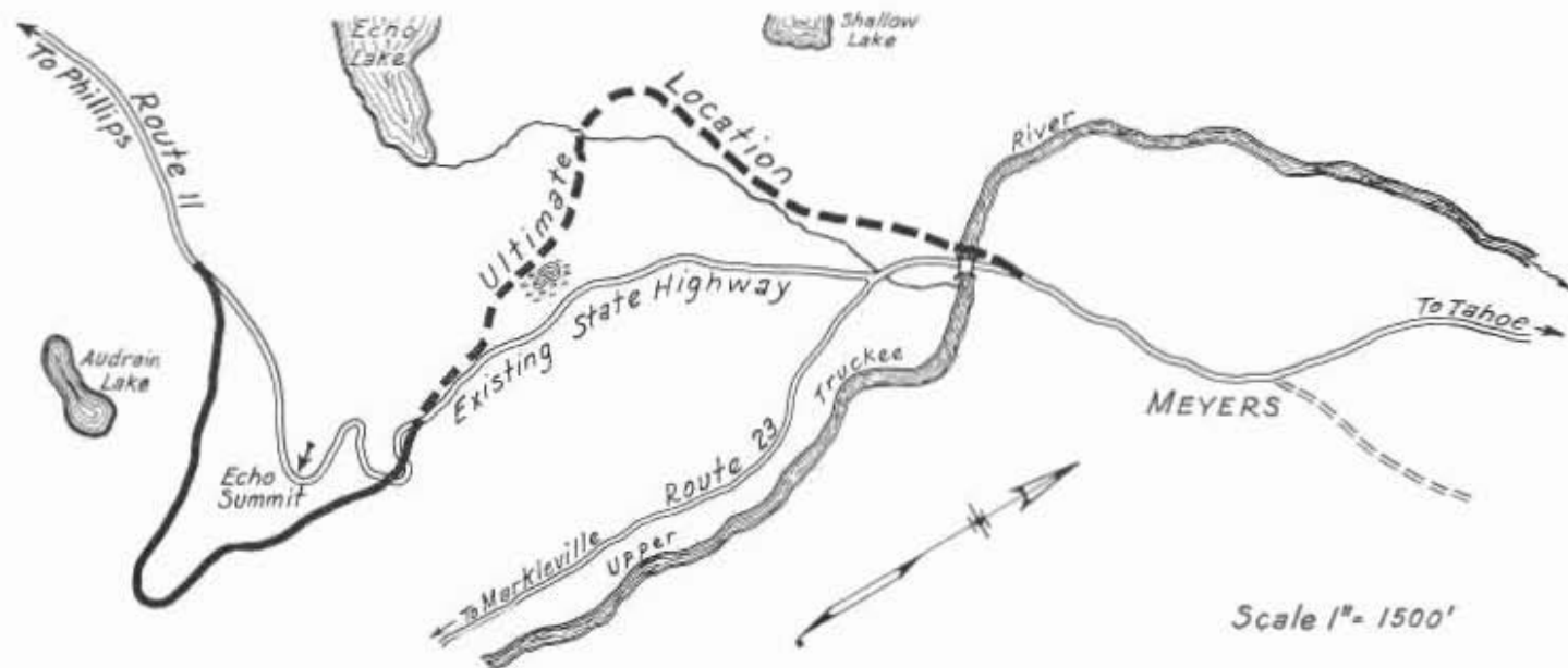
Black line shows newly opened sector at Echo Summit of Meyers Grade relocation on U. S. 50.
