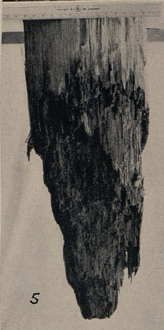
Typical ground line decay in untreated piles. The removed pile stub was rotted completely about two feet below the ground line as shown in Photo No. 5
