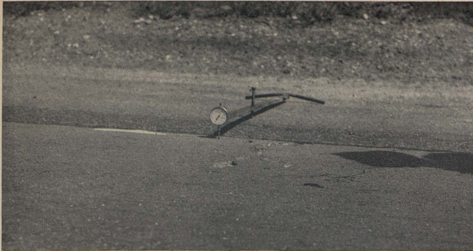
Ames dial used to record pavement rise in asphalt jacking (upper), and for measuring deflection of slabs (lower)
