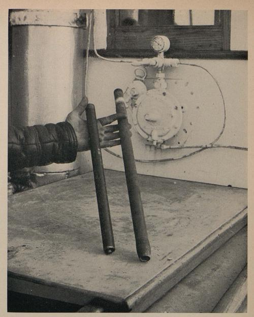
Sampler tips. Cutting point on right used for hard material
