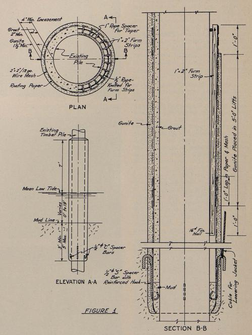
asphalt felt was laid over the form strips to act as the inside form. Wire mesh reinforcement, crimped to keep it off the felt, was then fastened in place over the felt. Two S-shaped hooks and guides were placed in the form, 180 degrees apart, and later cast in the concrete. Two C-shaped guides
