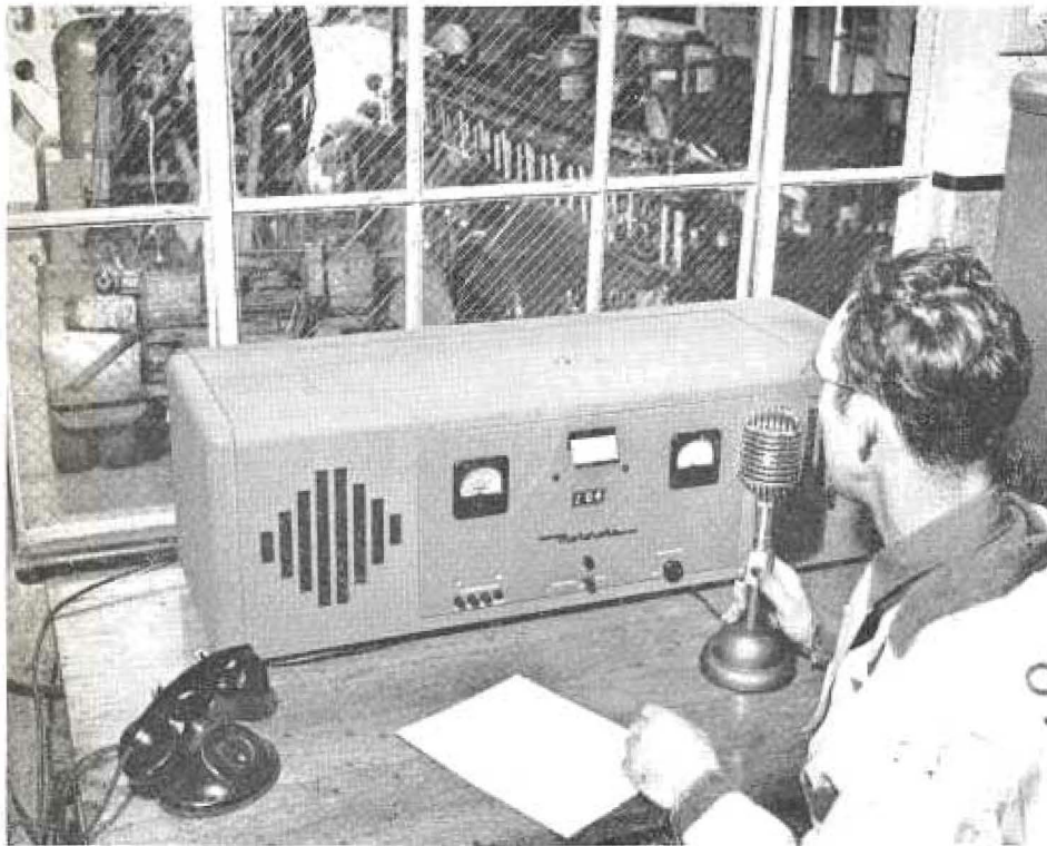
"Send Tow Truck," radios pickup truck operator on San Francisco-Oakland Bay Bridge. One minute later a tow truck arrived to haul away the car. Bridge traffic operations have been greatly expedited through the use of two-way FM radiotelephones
