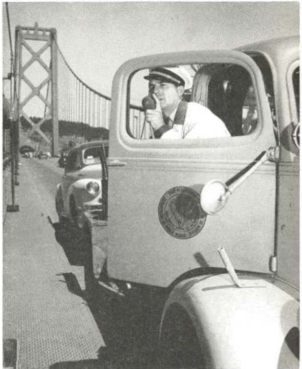
"Coming in with stalled car," radios tow truck operator on San Francisco side of San Francisco-Oakland Bay Bridge. Seconds count on this 6 mile long bridge where a car breakdown can seriously hinder traffic which averages 70,000 vehicles per day. A mobile two-way FM radiotelephone in the truck permits instant communication with the dispatcher
