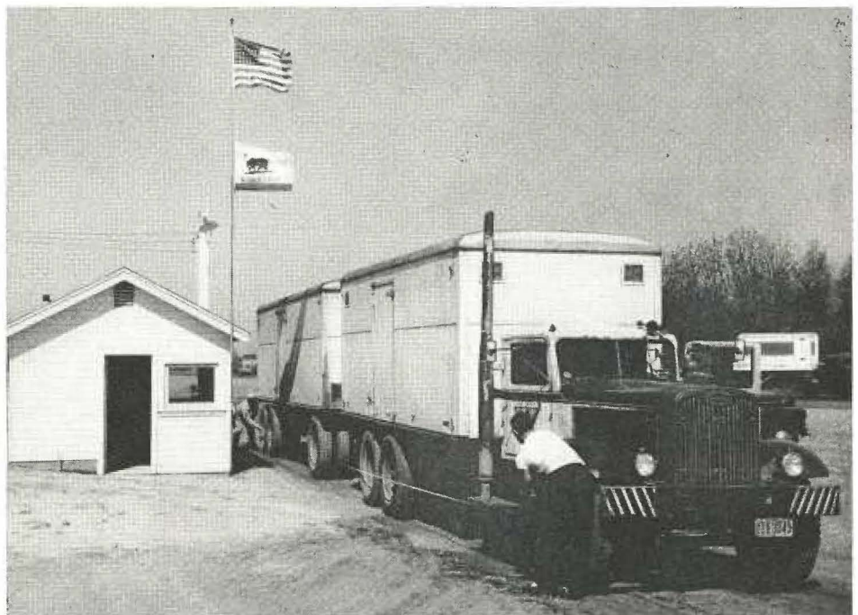
Measuring at Coyote to determine allowable gross weight. Note mast arm and height indication to right of flag pole
