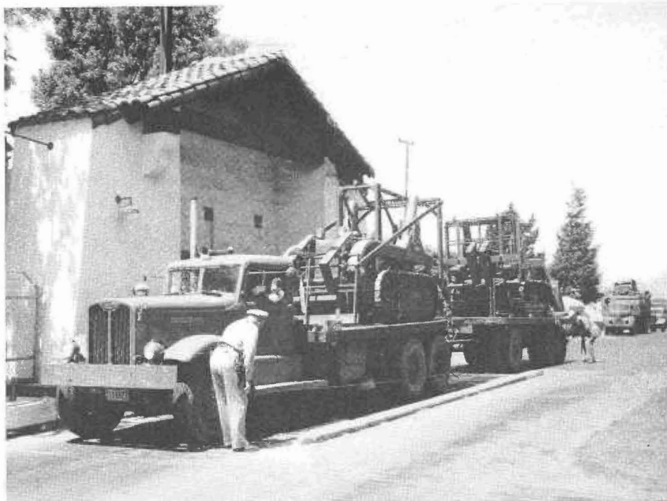
Truck-trailer combination being checked for gross weight and overall length at Carquinez Bridge scale
