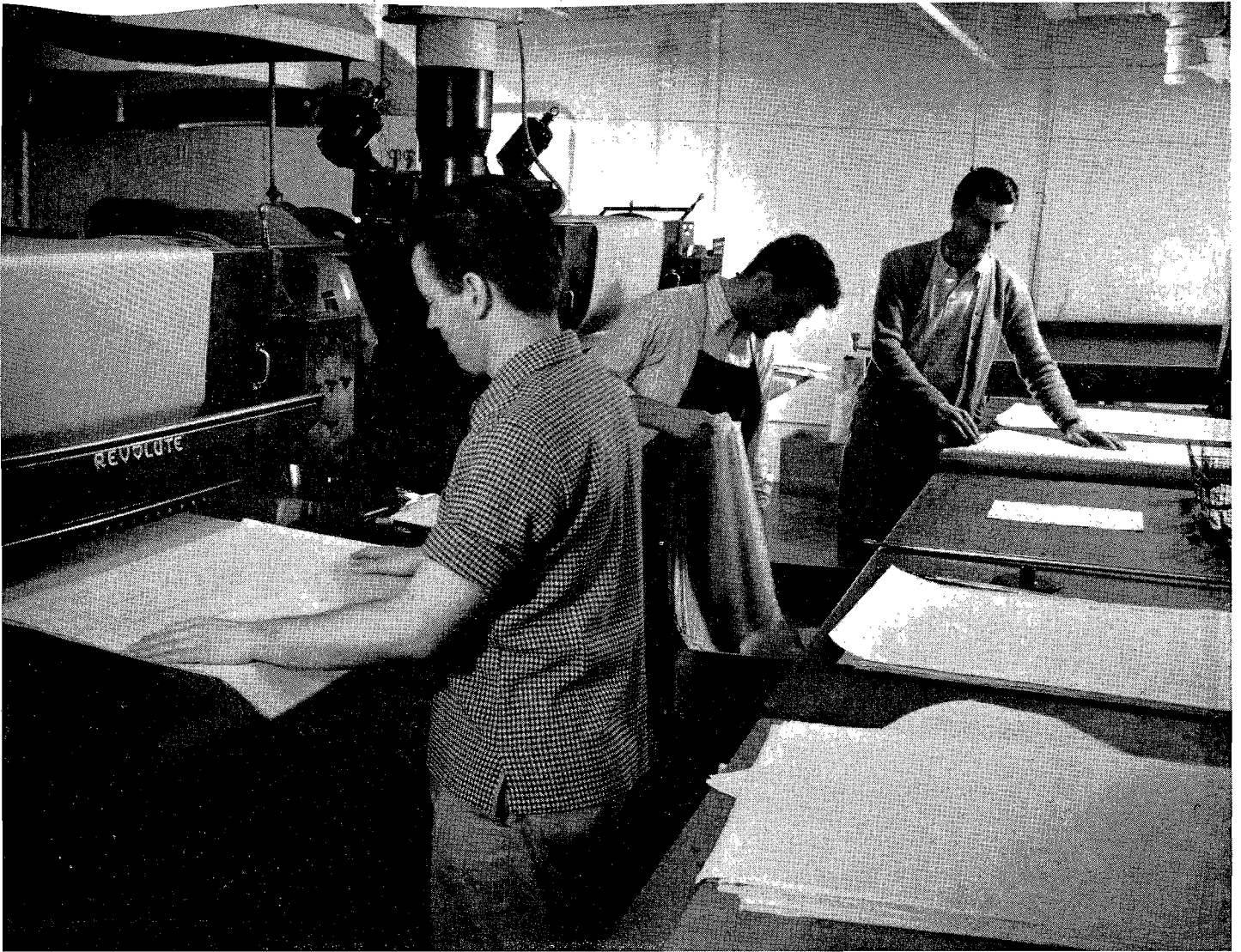
Feeding two continuous blueprint machines in Headquarters Reproduction Department. Machine in foreground running paper tracing at seven feet per minute
