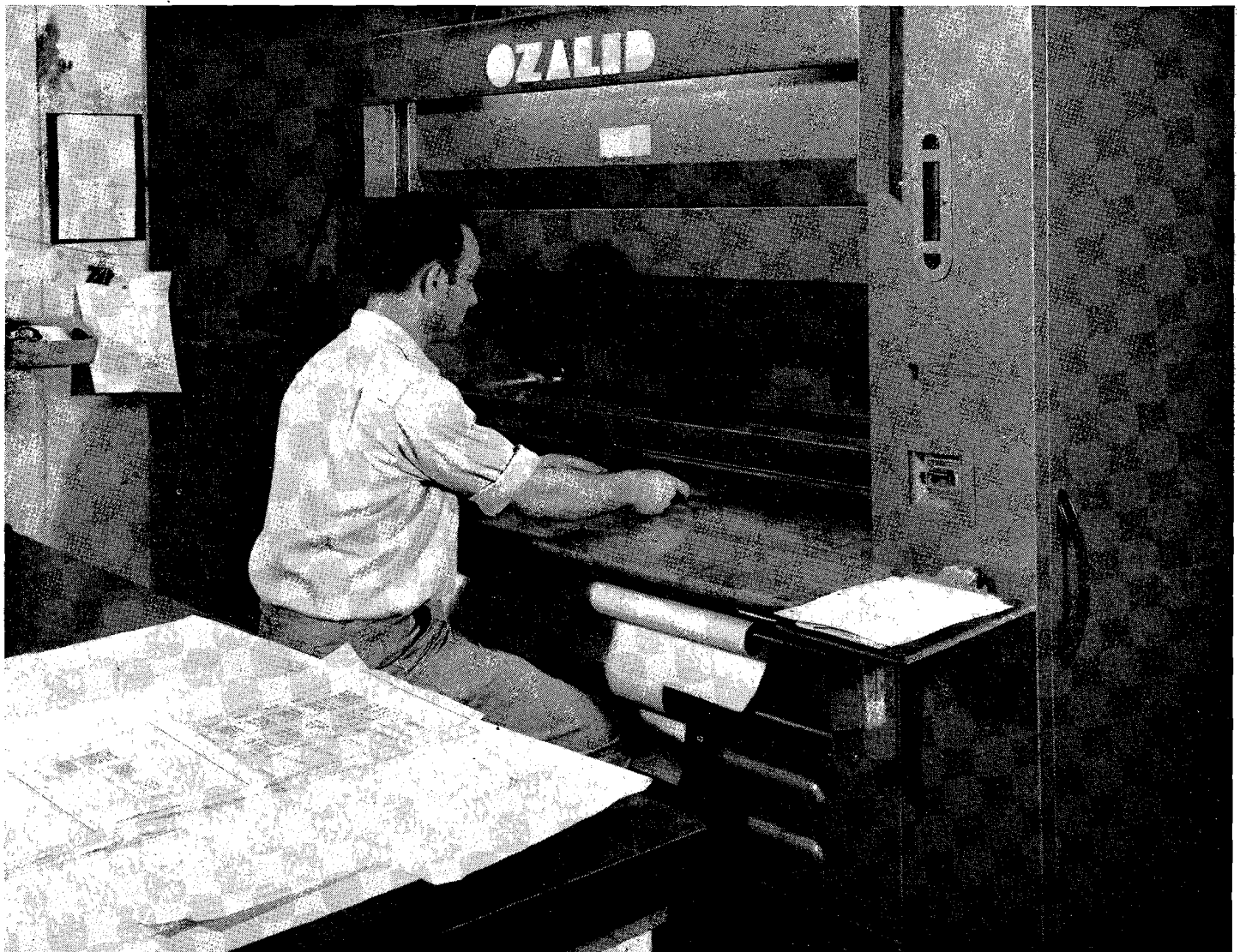
Operator feeding small paper tracings into continuous ammonia process printer in Headquarters Reproduction Department. Printing on cut sheets at 10 feet per minute
