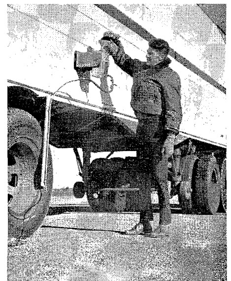
Apparatus used for making trace on pavement (Rear wheel of trailer)
