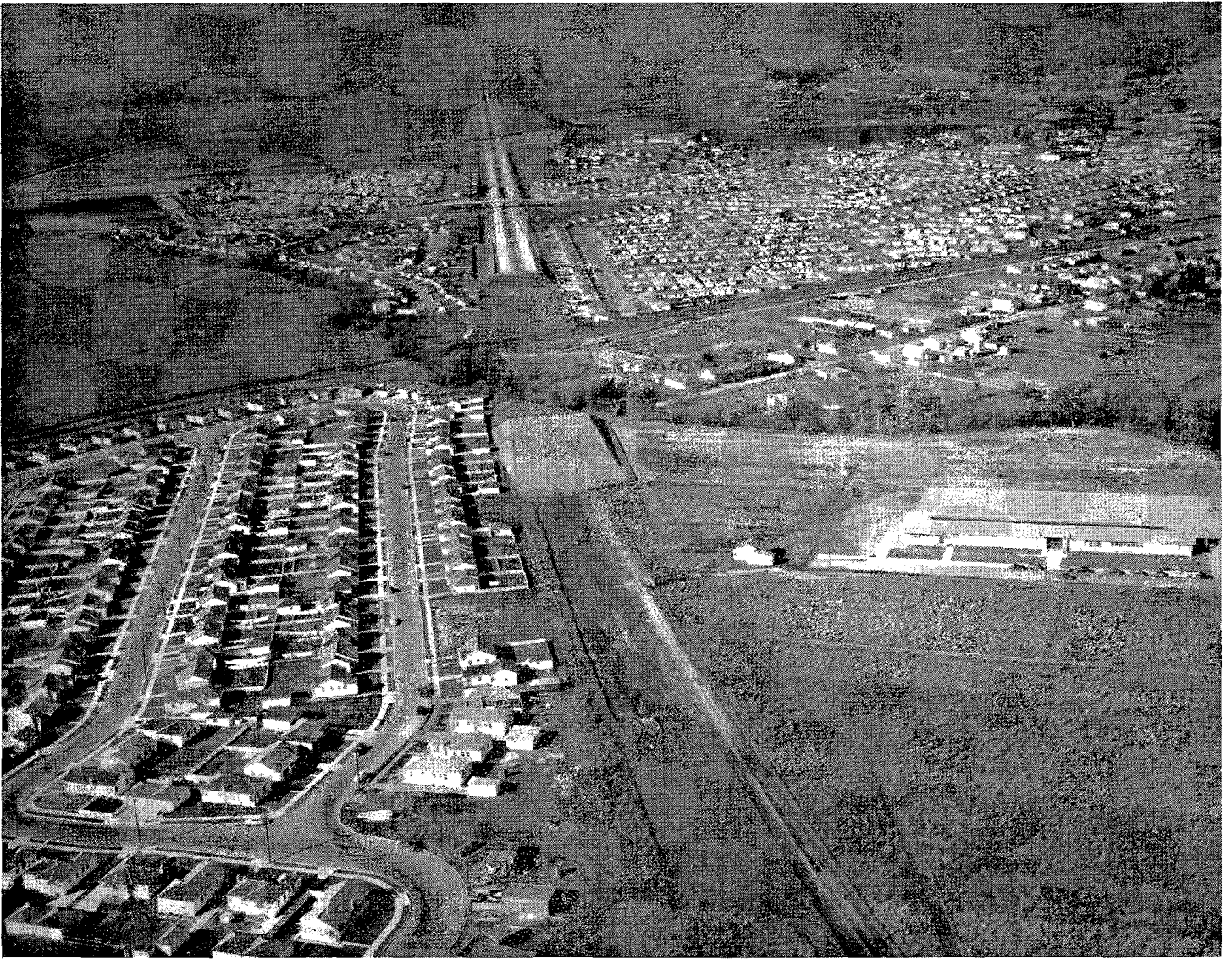
Air view northerly along East Shore Freeway from point near Davis Street, San Leandro, showing built up subdivisions on each side of the freeway right of way reserved several years ago when the residential development started, and now being utilized for the advancing freeway construction. Brookfield Village and the 98th Avenue and Hegenberger Road overcrossings show in middle distance, San Leandro Creek marking the southerly city limits of Oakland in center, and subdivision near Davis Street in near portion of picture
