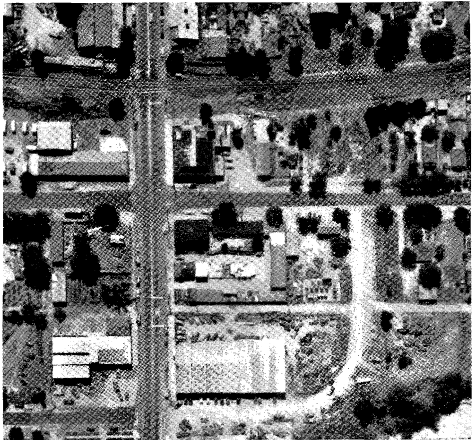
This vertical aerial photograph, supplemented by a relatively small amount of ground surveying, produced the contour map on the opposite page. Scale 1":400' on original photograph.
