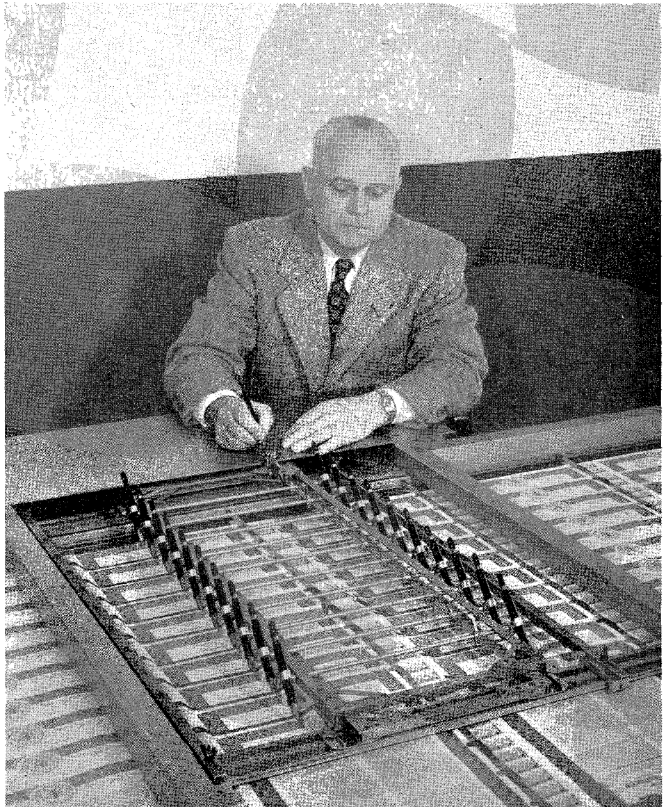
—→ This machine enabled Frank B. Durkee, Director of the State Department of Public Works, to sign 20 bonds at once for the $8,350,000 issue to purchase the San Mateo and Dumbarton bridges across San Francisco Bay. There were 8,350 bonds to sign and the machine cut the time for signing from a week to two hours.
