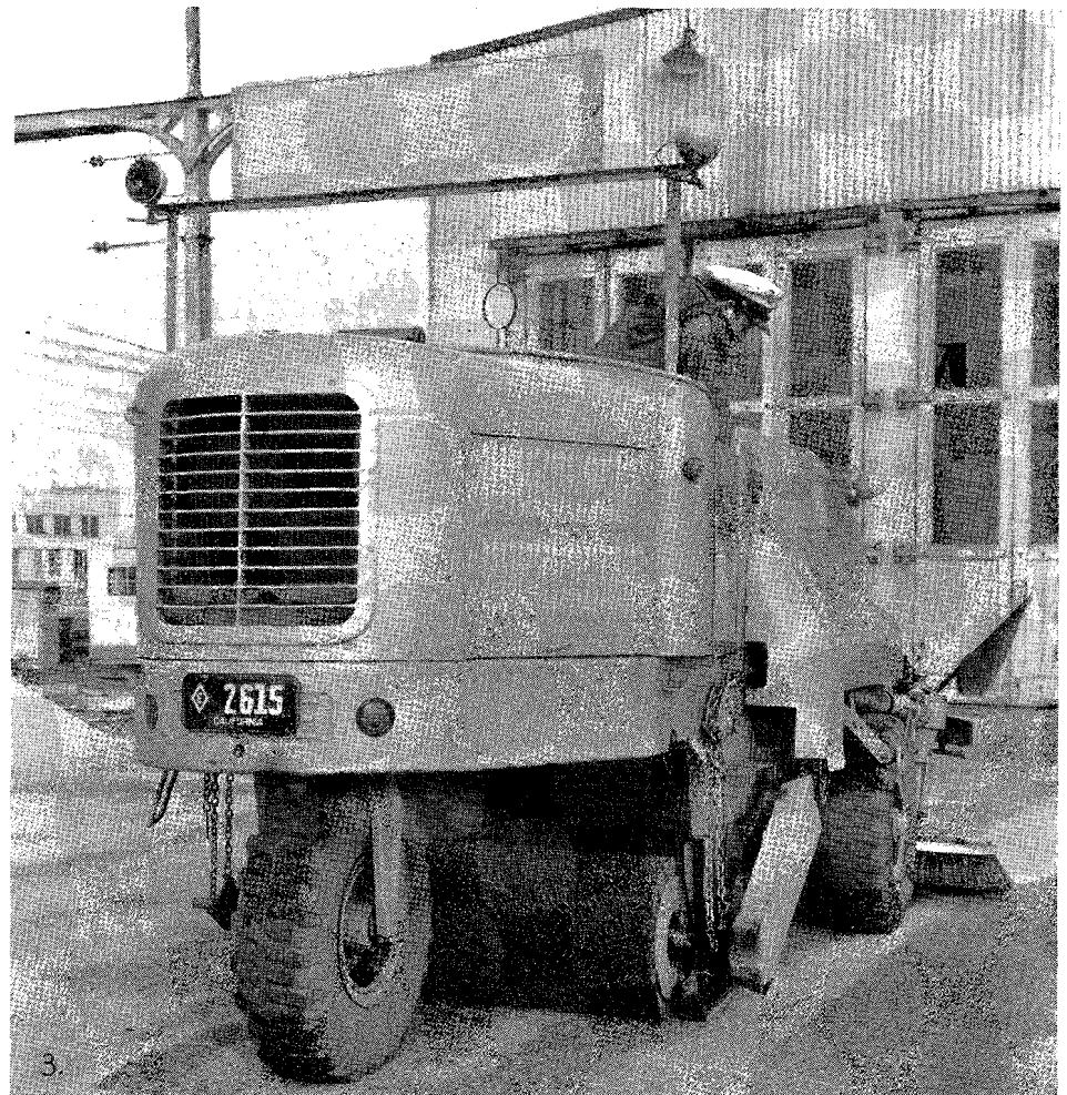
This is special power broom used on the San Francisco-Oakland Bay Bridge
