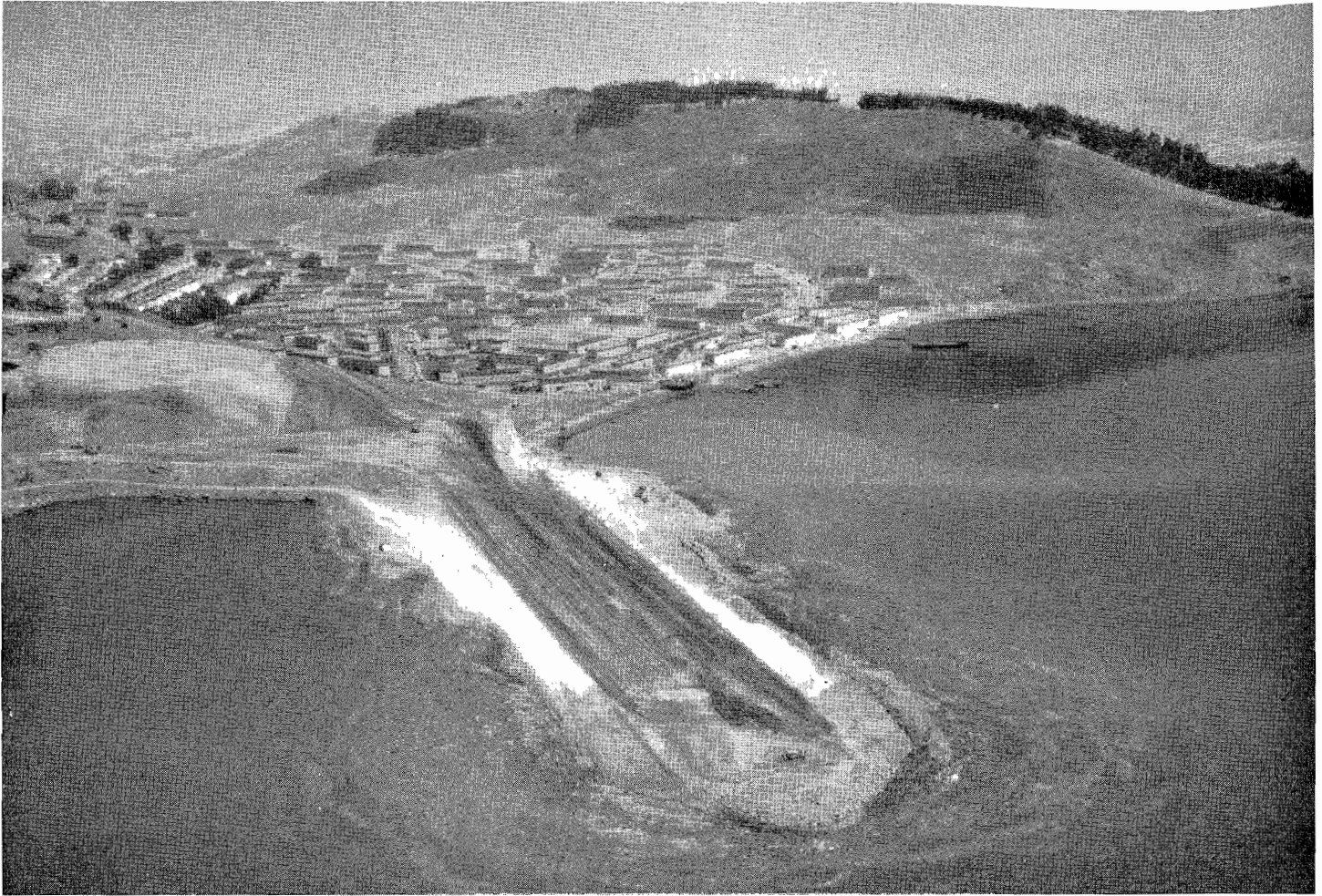
Aerial photograph of experimental fill looking north toward Sierra Point. Ultimate freeway alignment to pass through housing development and saddle in upper left-hand corner in photograph.
