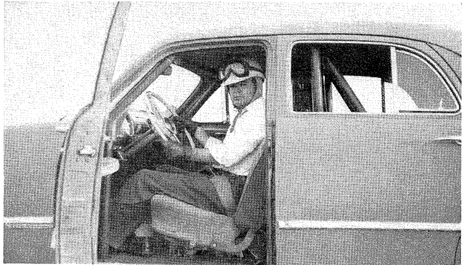
E. W. Kessinger, Test Driver, shows safety features of car. These include safety belt, crash helmet, welded pipe bracing back seat removed and front seat fastened down by direct ties to frame.
