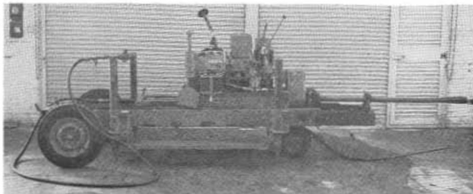
FIGURE 3 California horizontal drill with drill rod and bit in drilling position
