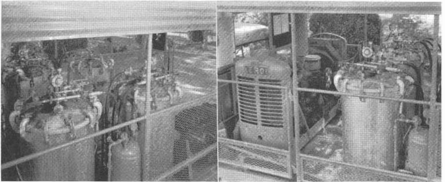
LEFT—Arrangement of paint tanks showing air driven mechanical agitators. RIGHT—Close up of compressor and paint tanks using air-driven mechanical agitator.
