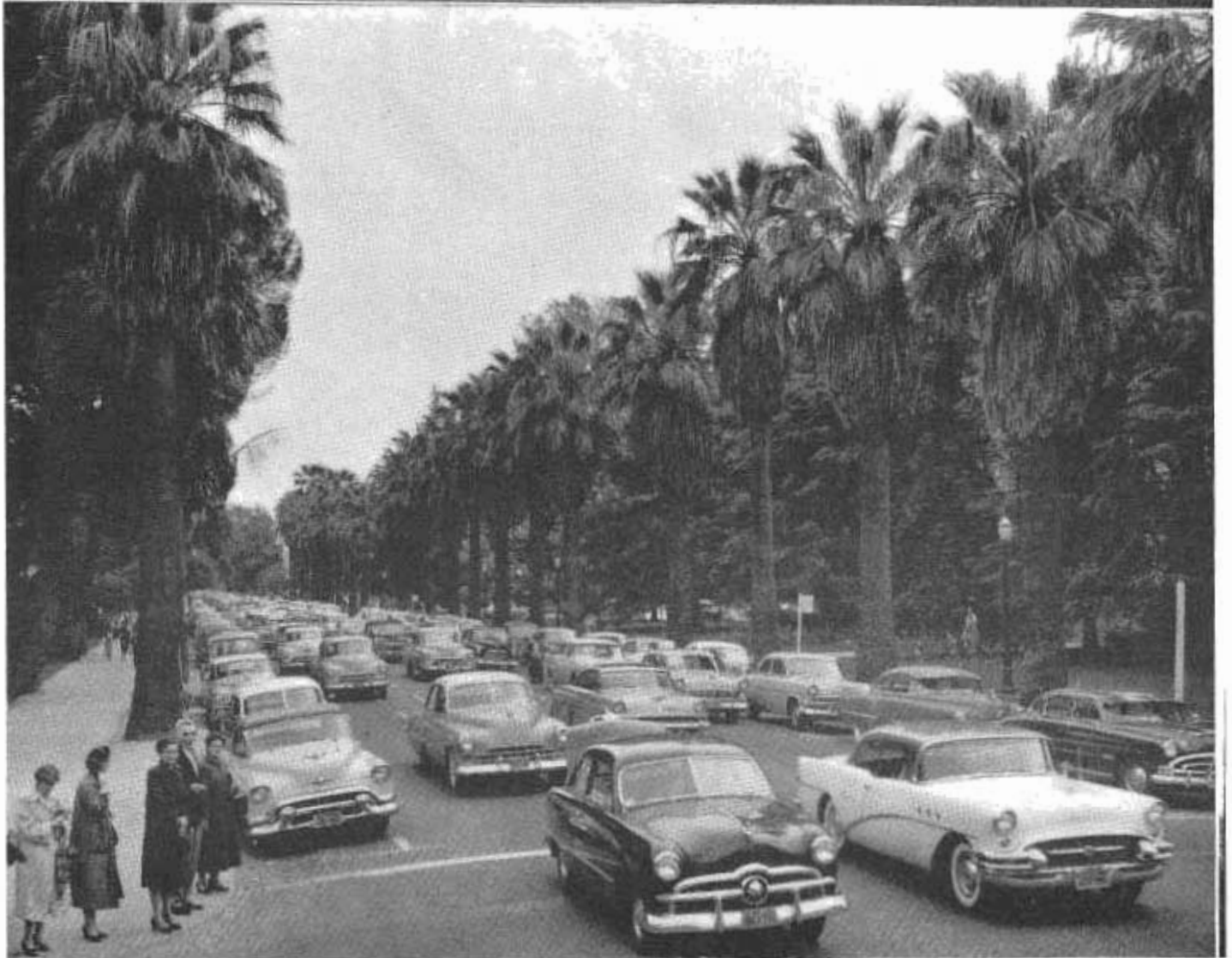
UPPER —Congestion is relative. At an intersection of two-lane highways with a capacity of 1,600 vehicles per hour, 1,800 vehicles per hour produced congestion. LOWER —At an intersection of three-lane, one-way city streets, capacity 2,000 vehicles per hour, an additional 100 vehicles per hour produced congestion.
