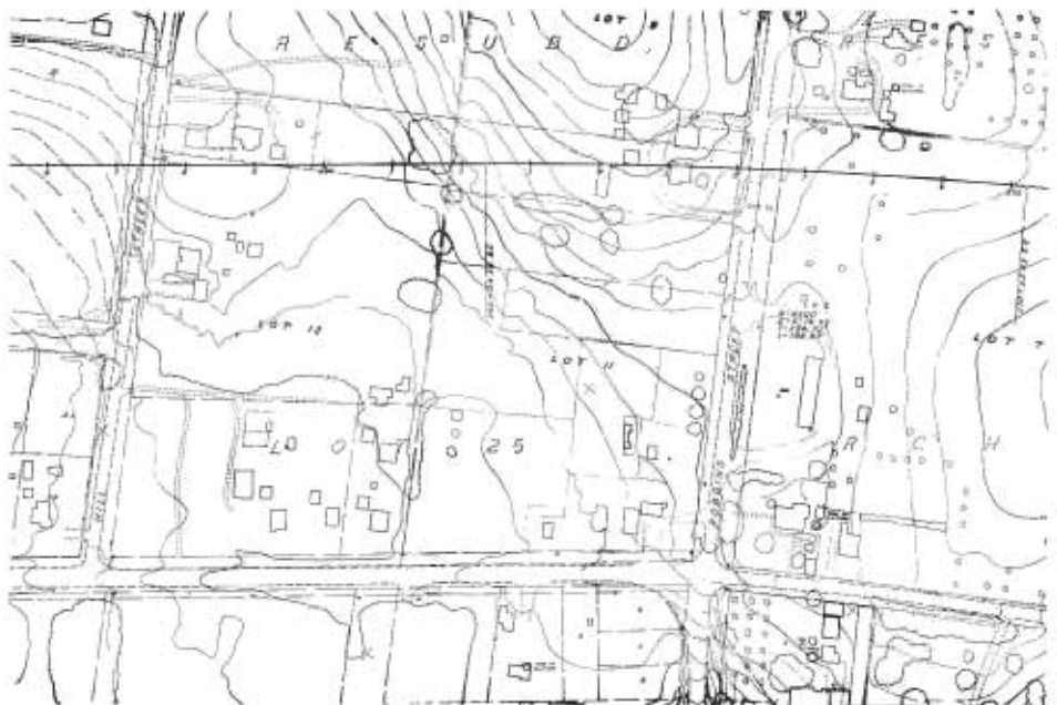
PHOTOGRAMMETRY —Above, a portion of an aerial vertical photograph taken along US 101 in southern San Luis Obispo County. Below, a corresponding portion of the detailed map which was plotted and drawn directly from the aerial photograph. The dark line running across the map near the top is the center line of the proposed four-lane expressway which will be under construction this spring. Modern photogrammetric methods drastically reduce the need for detailed ground surveys, thus saving many engineering man-hours for the Division of Highways in getting construction of modern highways under way.
