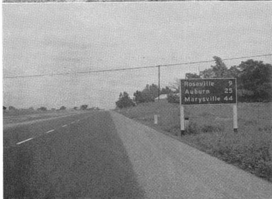
New type reassurance signs are larger and reflectorized for easy nighttime as well as daytime reading
