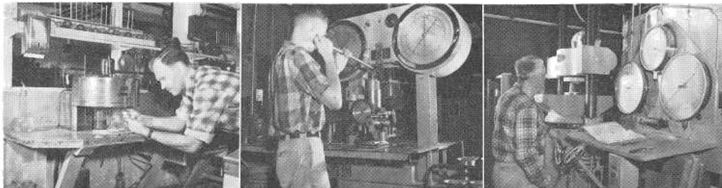
LEFT—Viscosimeter for determining grade of liquid asphalt. CENTER—Inserting test specimens in stabilometer prior to testing. RIGHT—Compression test for determining strength of cement-treated base test specimens.
