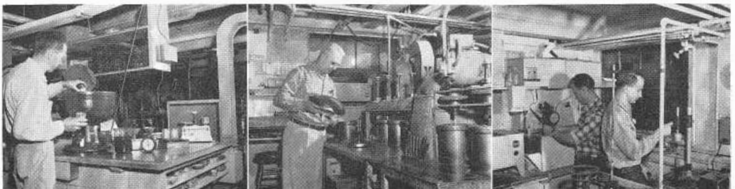
LEFT—Making centrifuge kerosene equivalent determinations in order to ascertain how much asphalt should be added to a paving mixture. CENTER—Mechanical mixer for mixing bituminous test specimens. RIGHT—Performing tests on bituminous products, penetration test for paving asphalts and shock test for pipecoating asphalts.
