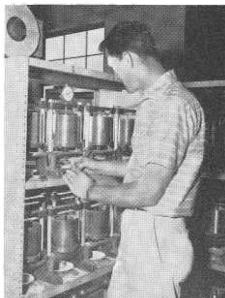
Small pressure tests to determine how much weight of base and pavement will be required to prevent soil from expanding
