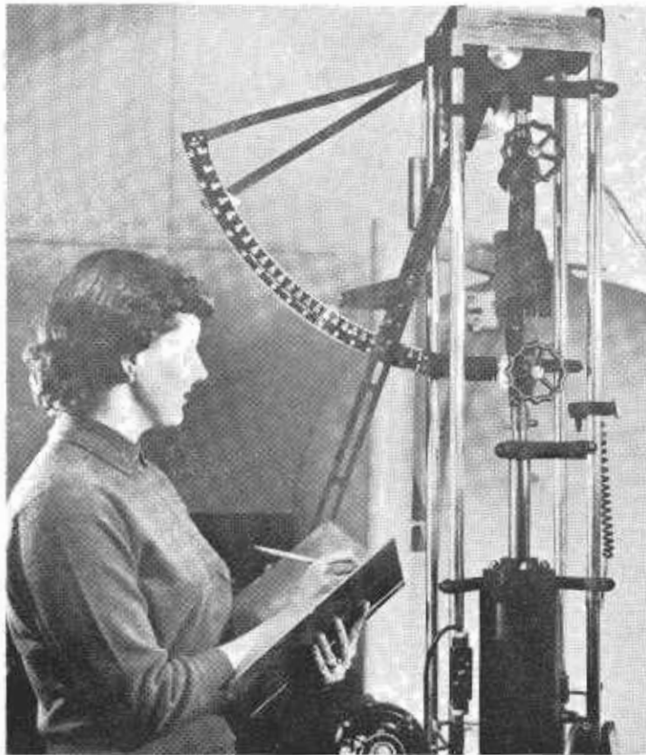
LEFT—Figure 10. Tensile testing of fabric material in an electrohydraulic tensile tester. ABOVE—Figure 11. Testing engineer and instrument maker are shown making final adjustments on a new type recorder designed and manufactured by the Materials and Research Department of the Division of Highways. Such combinations of precise machines and trained personnel have developed many special pieces of laboratory equipment.
