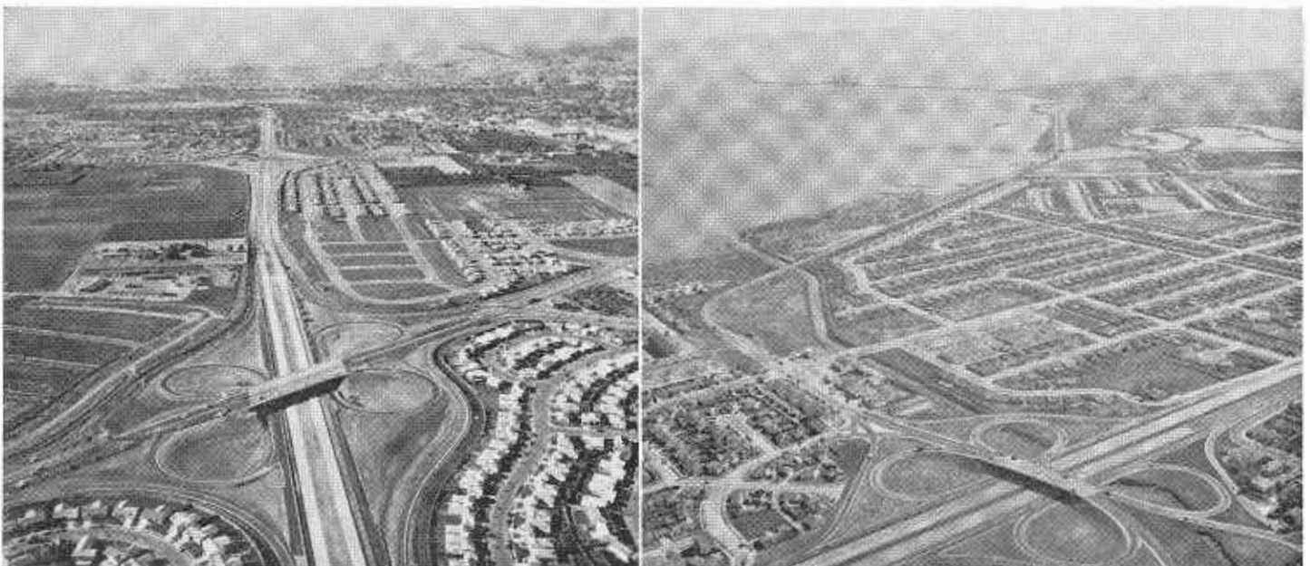
LEFT—Subdivision layout which provides for residences backing up to the freeway is described as more efficient than having homes face the freeway. The view is north along the Eastshore Freeway in Hayward, with the Jackson Street Interchange in the foreground. RIGHT—Aerial view of the Bayshore Freeway-Third Avenue Interchange area in San Mateo shows how a major artery (Norfolk Street) makes for good local traffic movement in a subdivision.
