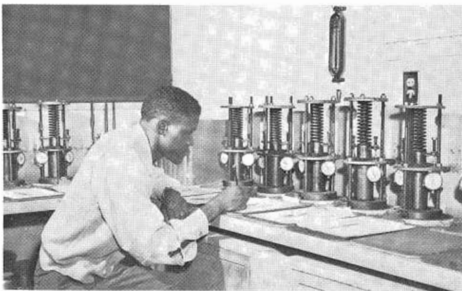
Reading spring-loaded consolidometers to obtain test data used for estimating settlement
