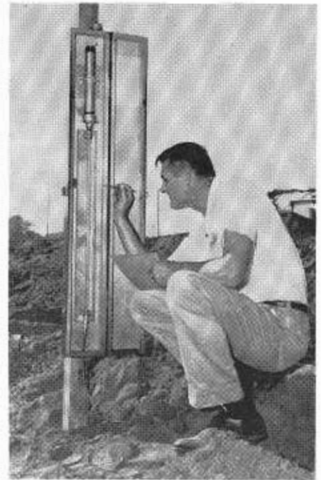
Reading settlement of ground beneath the weight of a fill by means of California designed settlement measuring device
