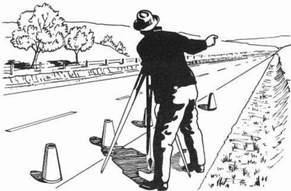
Members of survey parties working on any portion of a highway wear a red shirt, poncho, vest or coat. These may be luminous or standard cloth.
