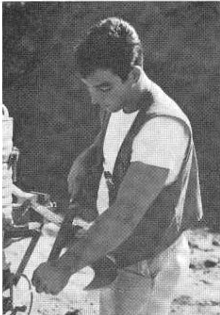
A member of a survey crew demonstrates a safe method of sharpening the blade of a brush cutter with the handle held in a vise.
