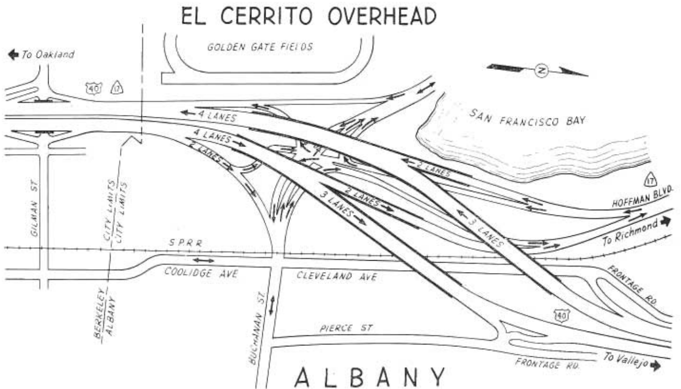
The arrows on this diagram of the new El Cerrito overhead show the direction of traffic flow on the main roadways and ramps.
