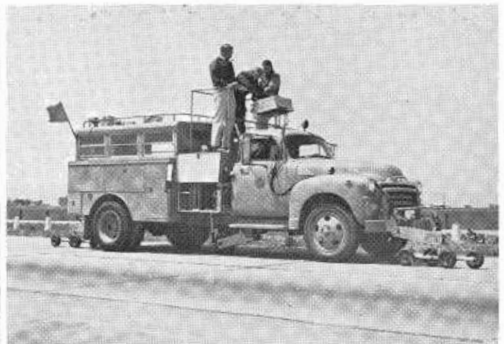
FIGURE 23—The profilograph in Figure 22 showing the recording console in the elevated position.
