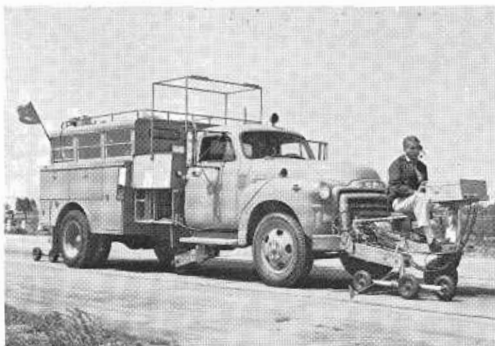
FIGURE 22—A mobile profilograph constructed by the California Division of Highways in 1955 showing the operator in position to record cracks and joints.
