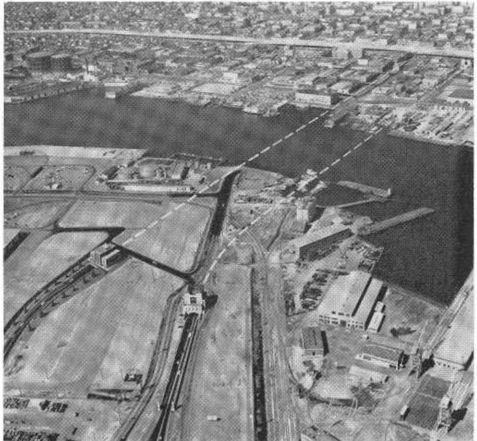
Retouched aerial photograph of project site. Dotted line on left shows location of Webster Street Tube. Existing Posey Tube is indicated by dotted line on right.
