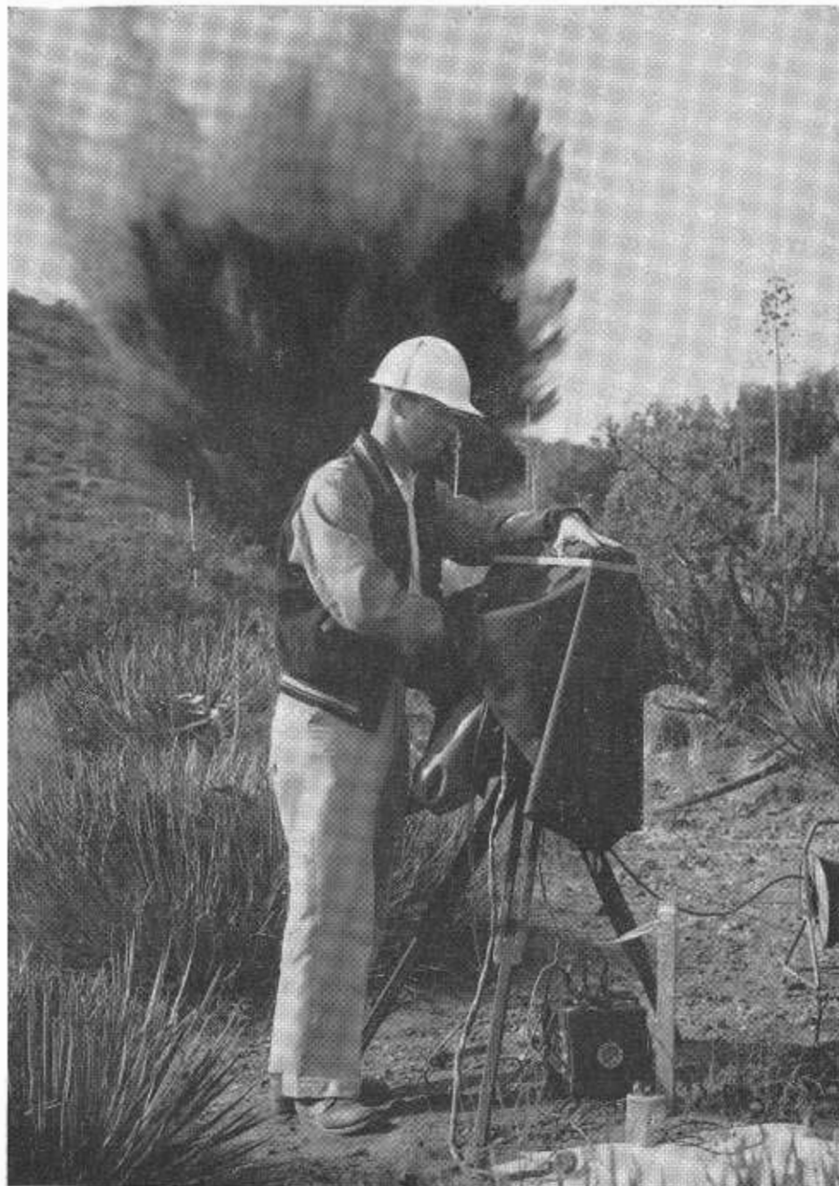
Marvin McCauley sets off a shot point for a seismic record.
