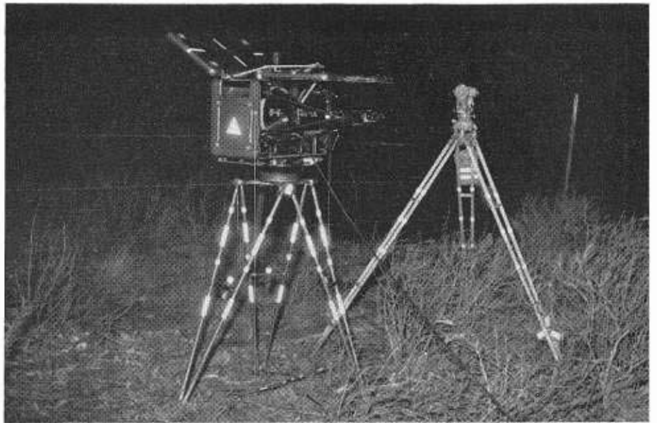
To the left is the master unit ready for observations and measurements. To the right is the theodolite to measure the horizontal angles between stations being observed.
