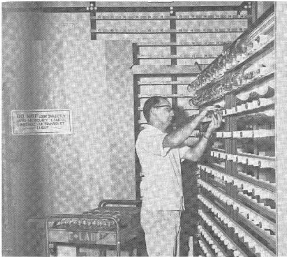
All materials used in highway construction are subjected to rigid tests to make certain the state's high standards are being met. Even incandescent globes (above) used in signal lamps must undergo the scrutiny of department technicians.
