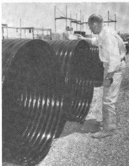
Bituminous-coated corrugated metal pipe is inspected prior to shipment.
