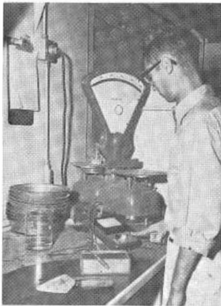
FIGURE 5. Measuring the minimum electrical resistivity of soil at any moisture content. This resistivity value of soil is used for estimating perforation time of metal culverts.
