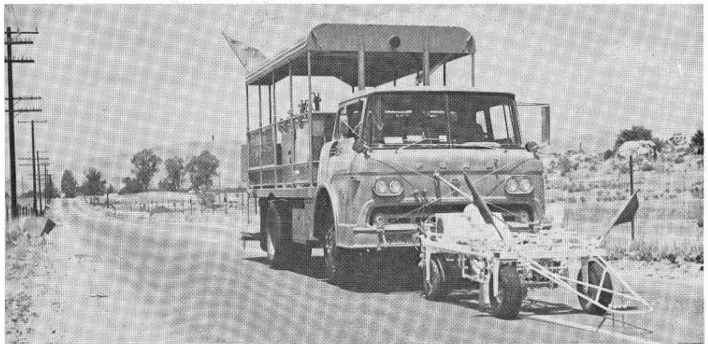
This high crown secondary road presents no problem to the new striper with its narrower tread.
