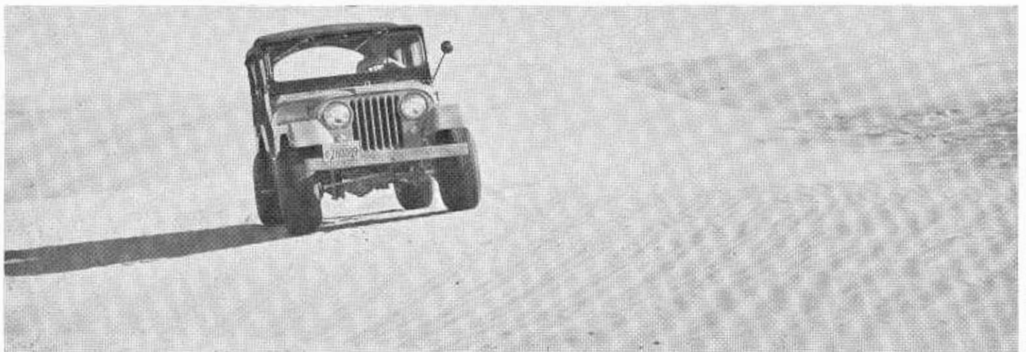
This Division of Highways jeep is equipped with large tires for driving on the sand dunes.
