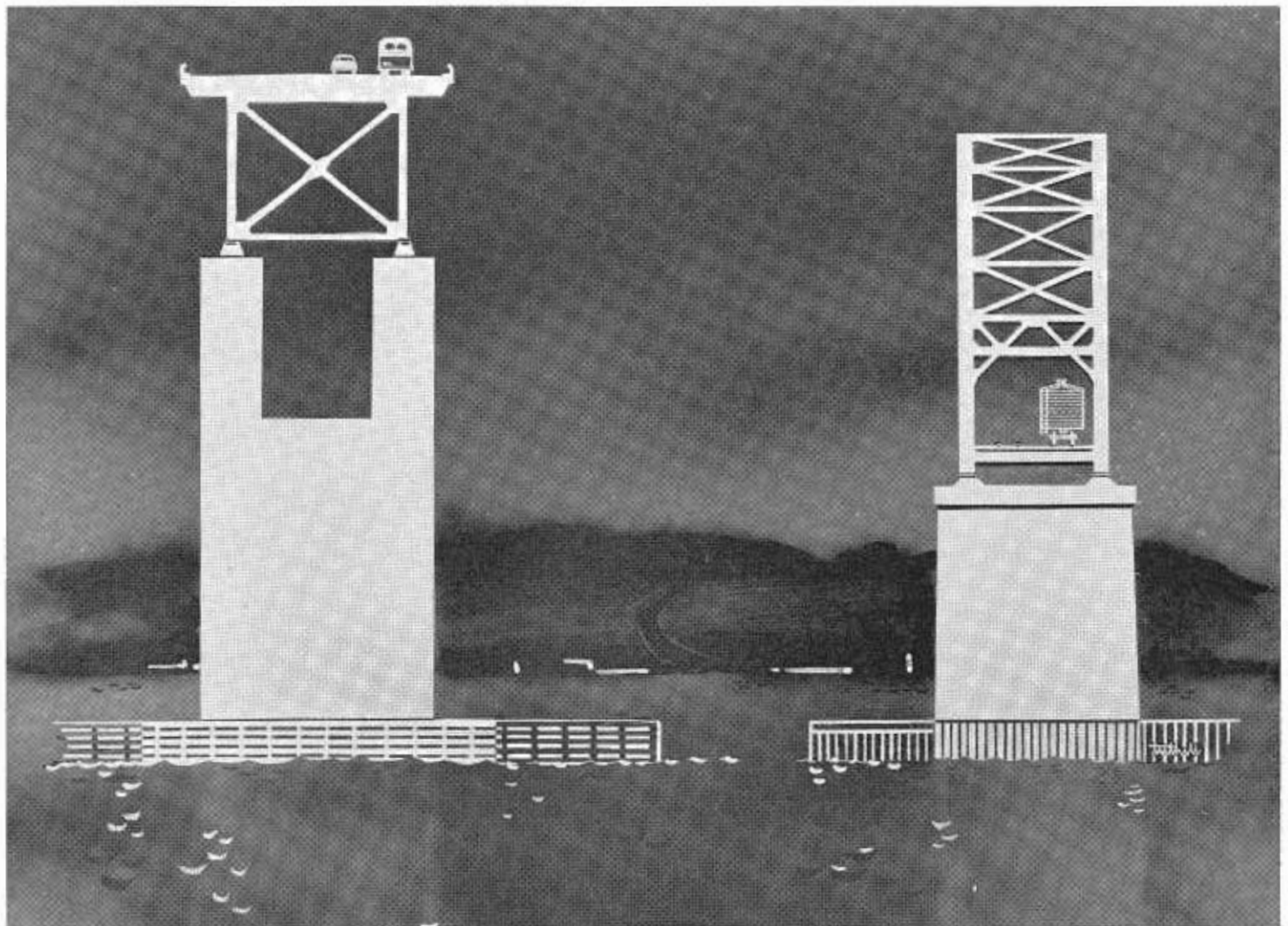
This sketch shows the relation of the new highway structure to the existing Southern Pacific Co. Bridge and the relative height of the highway deck above the water level. Maximum vertical clearance at the navigation channel between low steel and water is 138 feet on the highway bridge and 70 feet on the railroad bridge. The railroad bridge requires a vertical lift span for the passage of river traffic. Highway traffic will be about 178 feet above water at the highest point.
