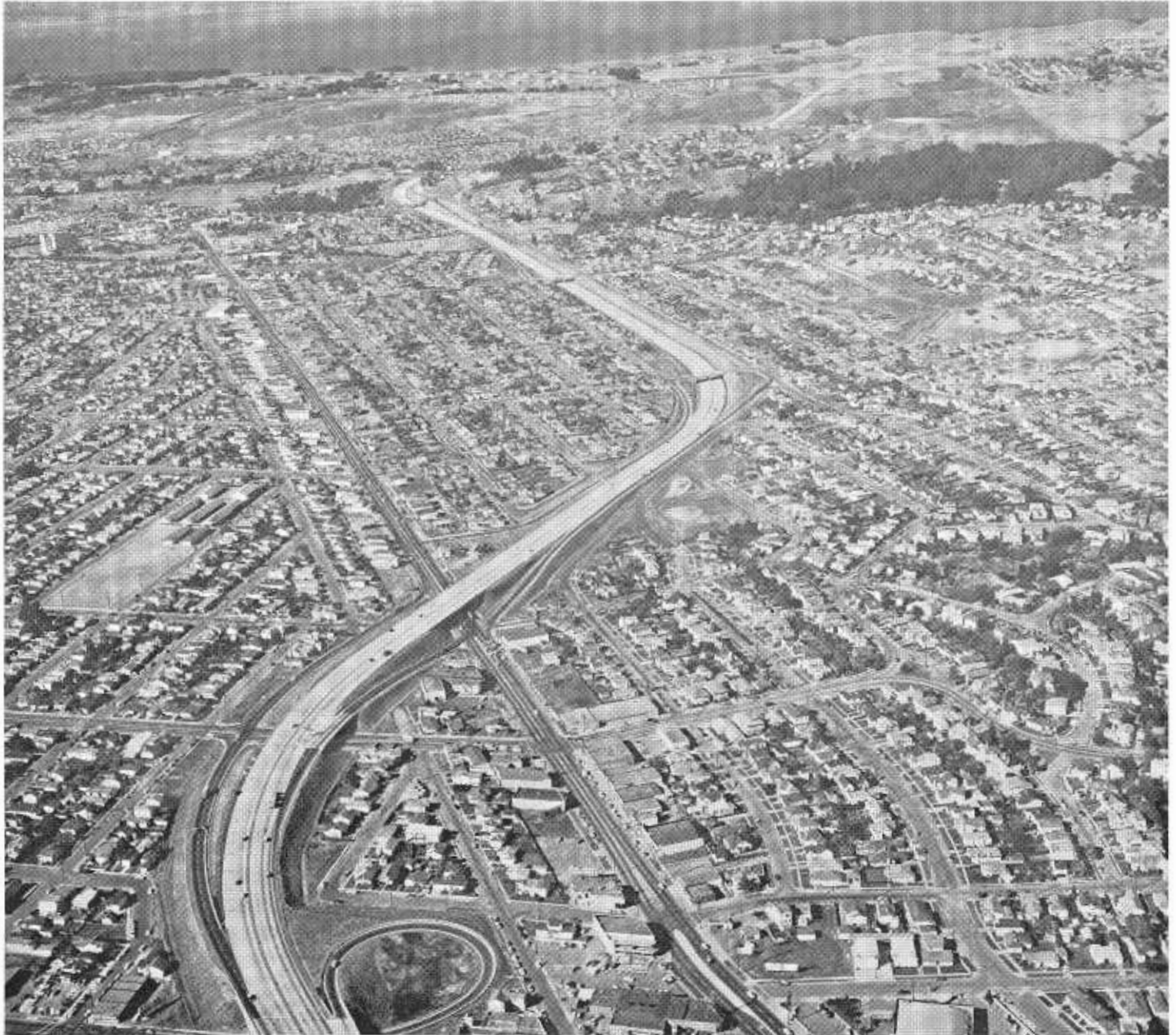
A typical portion of a constructed freeway through a metropolitan area, in this case U.S. 40 through Richmond. To provide adequate traffic service to commercial, industrial and residential areas, many streets must be served to and from the freeway. This illustrates the need for proper planning since the design of one interchange is dependent upon the design and proximity of adjacent interchanges.
