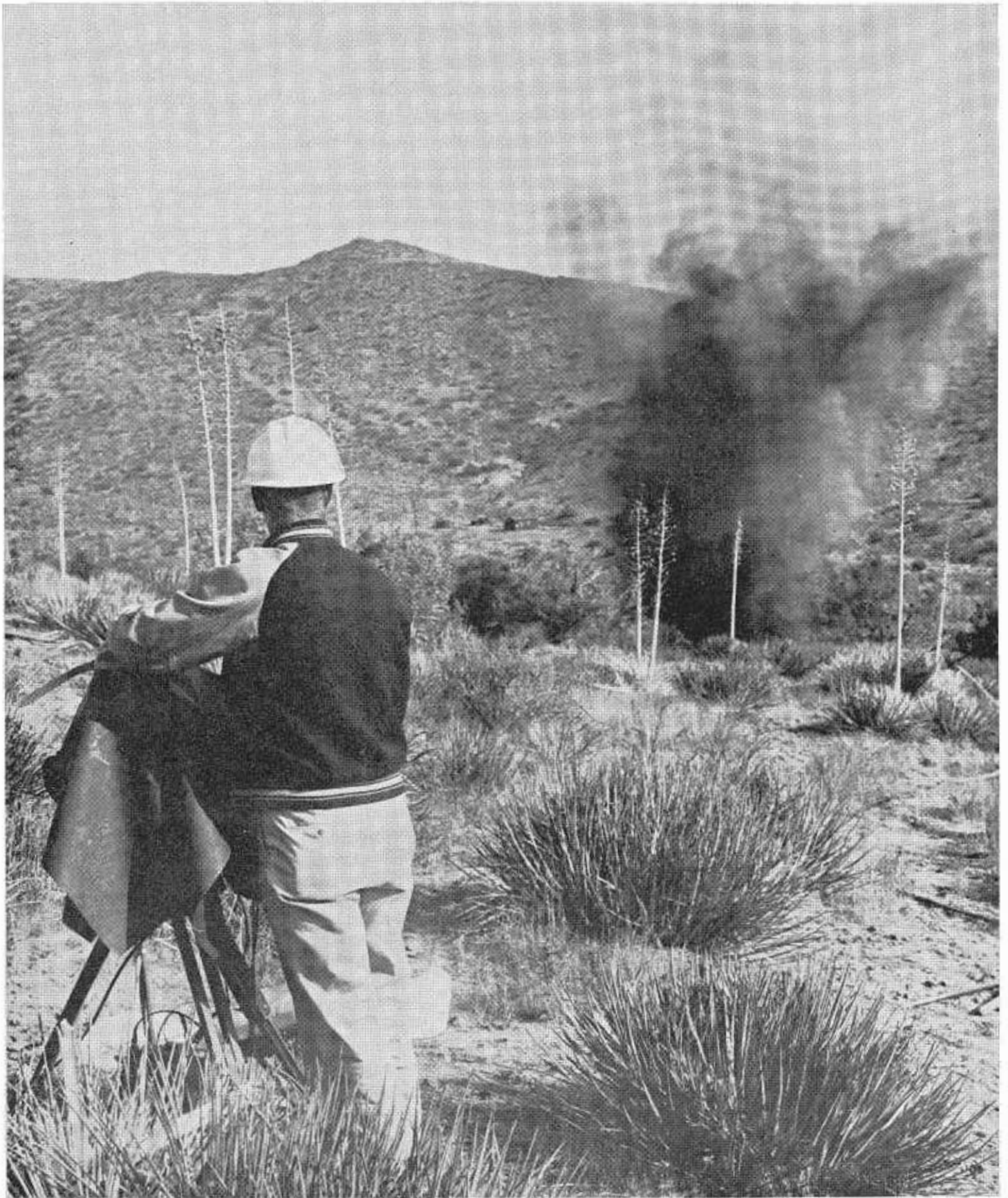
Blasting in connection with a geological investigation using a refraction seismograph.
