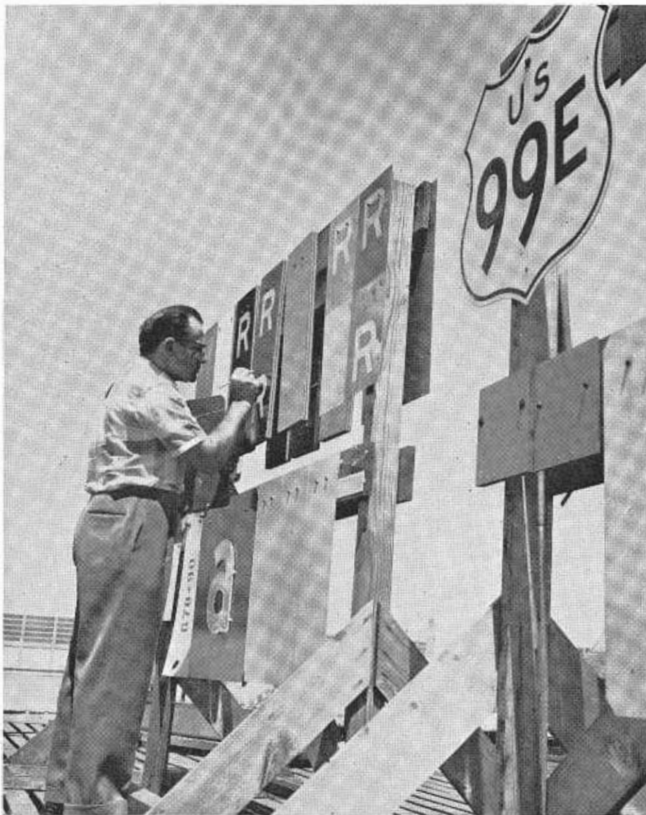
Exposure racks are used to test durability of signs and sign materials under the state's varying climatic conditions.
