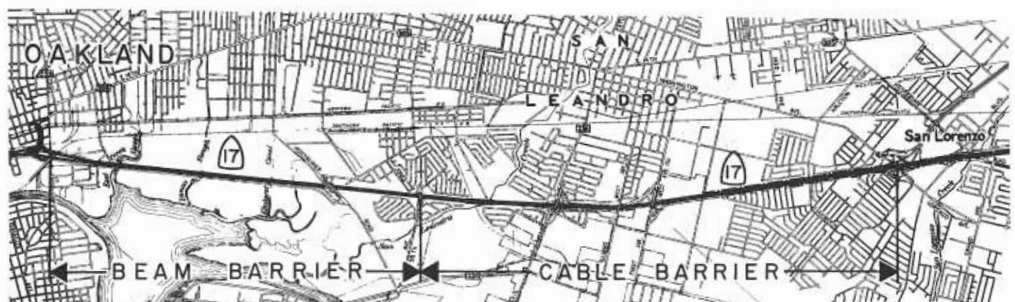
A map of the test section on the Nimitz Freeway in Alameda County where 3.87 miles of cable barrier were erected end-to-end with 2.87 miles of beam barrier.
