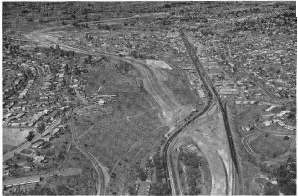
An aerial view looking northeasterly along realignment from Grossmont Summit where new freeway gradually drops to valley floor. Black road is old highway which goes through center of city.
