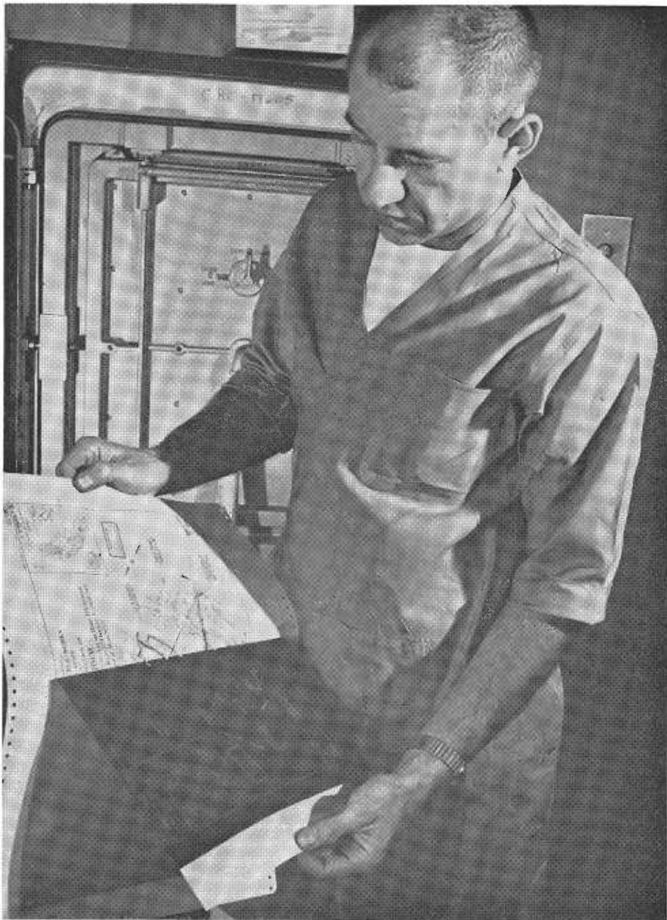
Reproduction Machine Operator Donald Geiger demonstrates the transferring of a plan image to an offset paper master.
