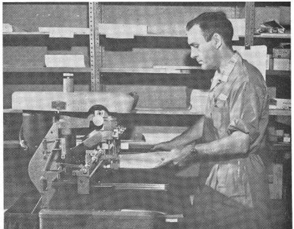
A completed set of plans is being punched on a multiple-head drilling machine by operator Charley Reynolds.
