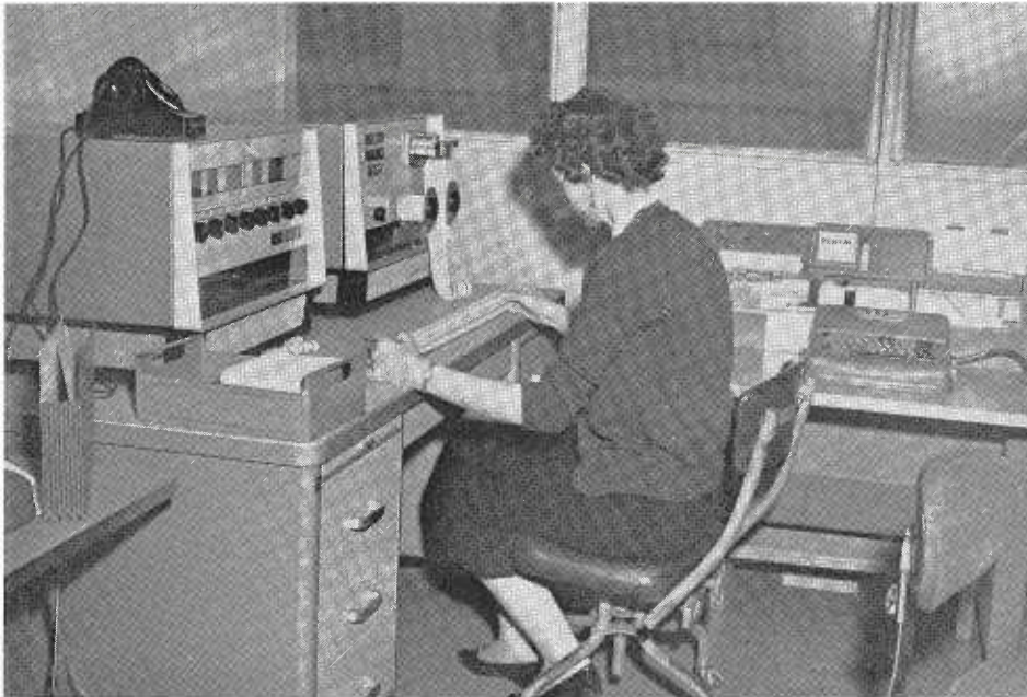
This two-unit automatic traffic tape translator is connected to the keypunch machine in the background. It transfers the hourly data to punched cards for machine listing and further processing.
