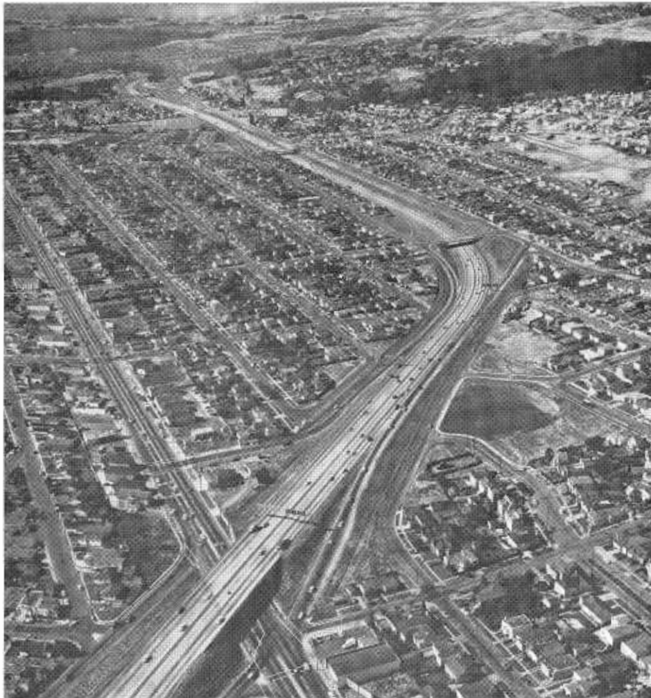
Looking north from San Pablo Undercrossing in Richmond, showing the modern interstate facility which replaced the old route with its many signalized intersections (left).
