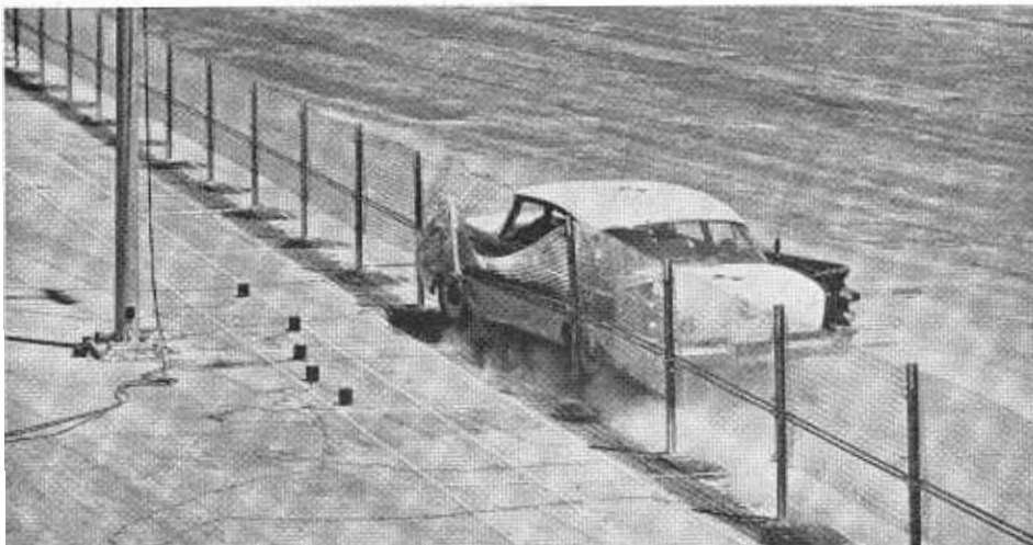
A test car crashes into the new design cable-chain link barrier at 75 miles an hour. Note the lack of rise of the front of the car during this flat angle collision.
