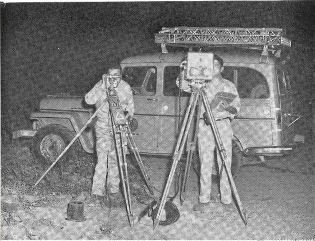
Typical operational set-up at night; Dan Radmanovich at the Geodimeter, Lee Winn measuring the vertical angle with theodolite.
