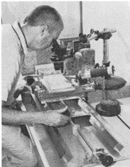
Linear traverse device used in determining the entrained air content of hardened concrete.
