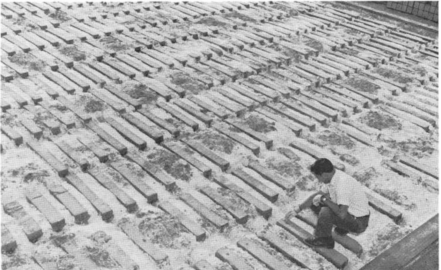
An inspector checks concrete beams, which have been subjected to wet and dry cycles and long-term exposure in soils containing high percentages of sodium sulfate. The beams, tested in co-operation with the Portland Cement Association, have been in the "duck pond" since 1945.
