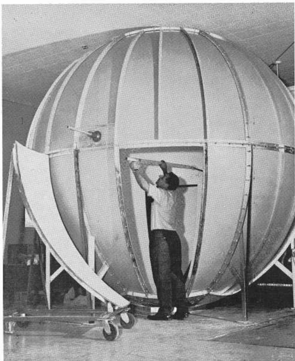
A fluorescent lamp being installed for testing in the integrating photosphere. The sphere is quite unusual, as there are only two or three others in the country which approach this unit in size.
