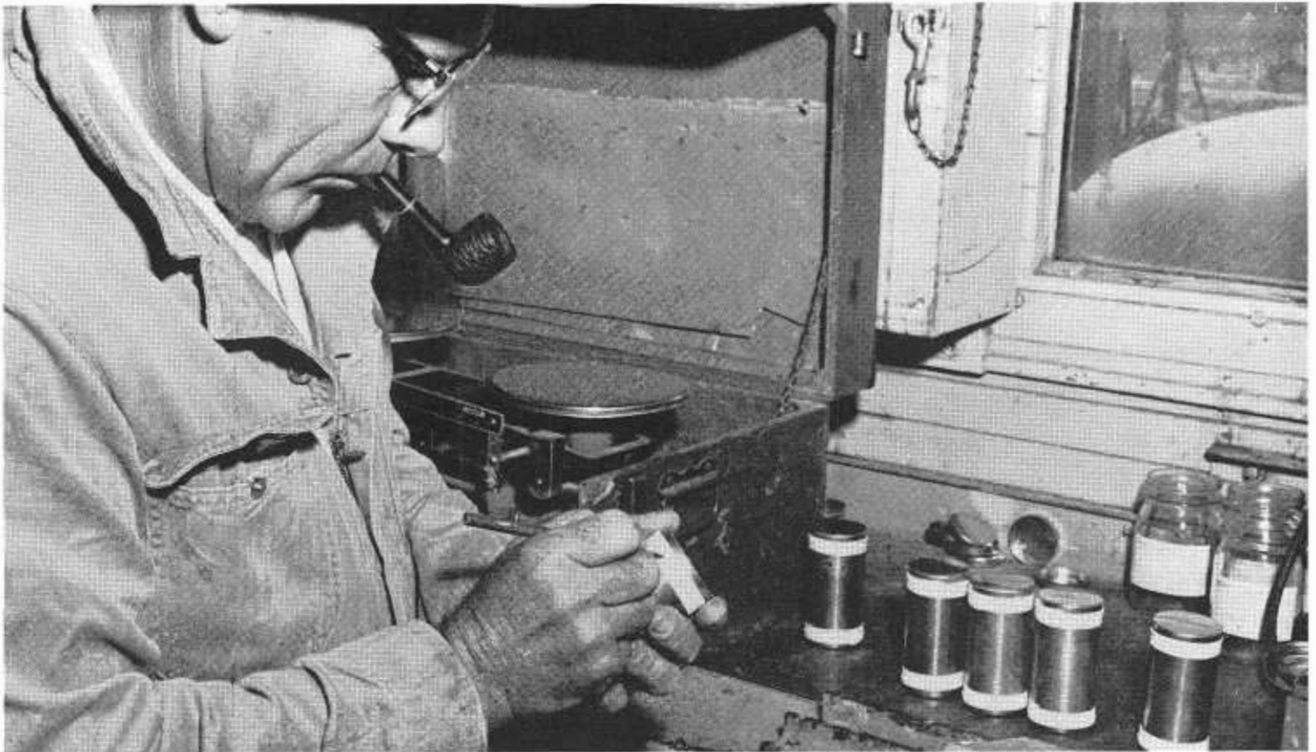
"Undisturbed" tube samples of soil are carefully sealed and labeled in the field for shipment to Headquarters Materials and Research Department Laboratory.
